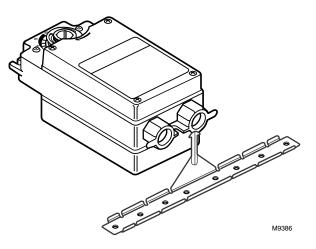
Fig. 2. Installing mounting bracket on ML6275 Direct Coupled Actuator.
